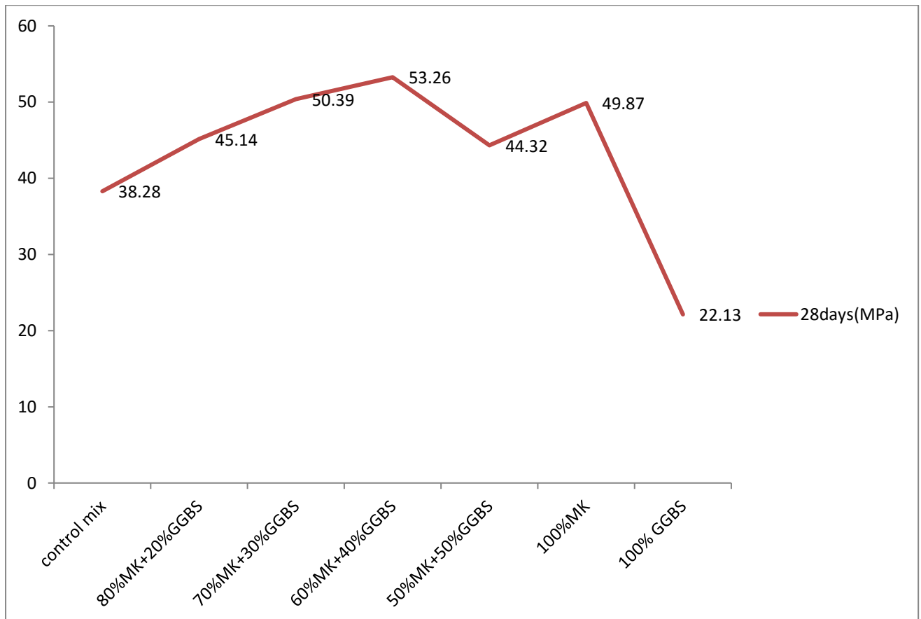
Figure 8 Compressive strength of Geopolymer concrete for 28days
